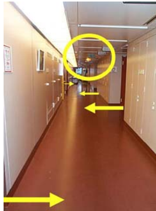
Fig. 11. Architectural space vs. escape signage.
